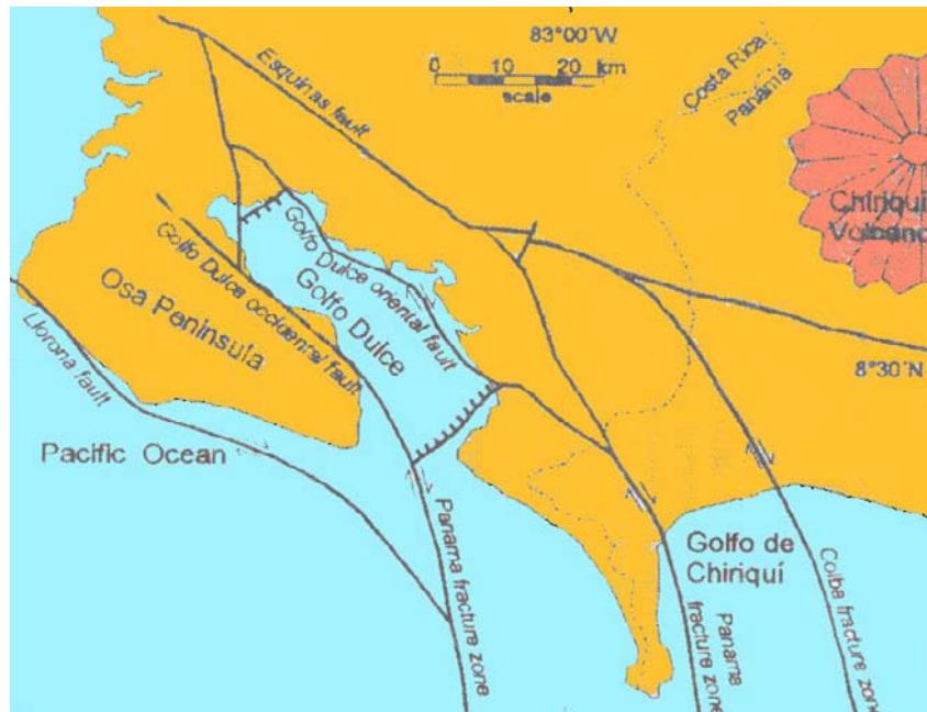
Figure 2.2 Tectonic fault systems in Golfo Dulce (simplified from Berrange 1989)
